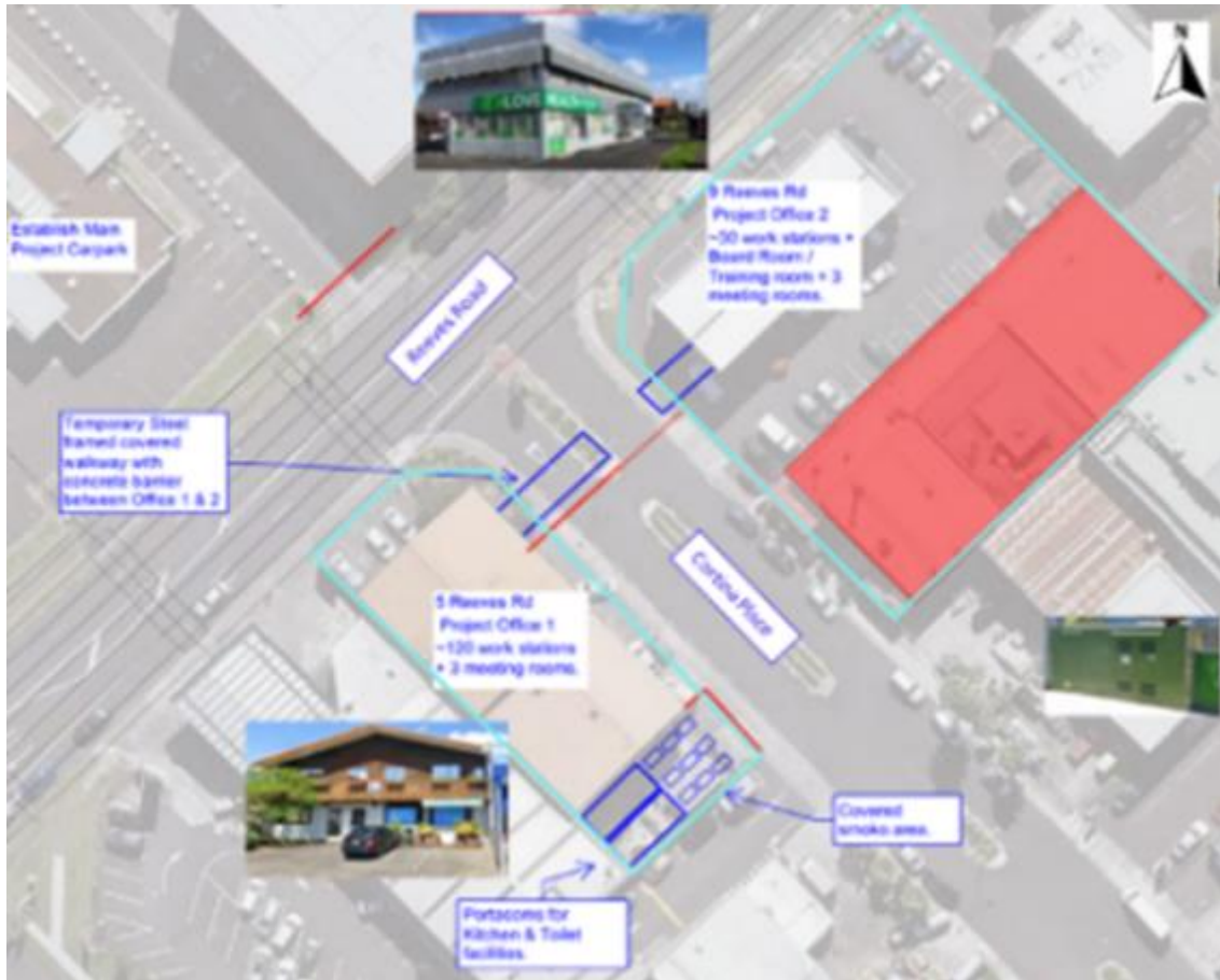
Figure 50: Site Office 1 and 2 locations
