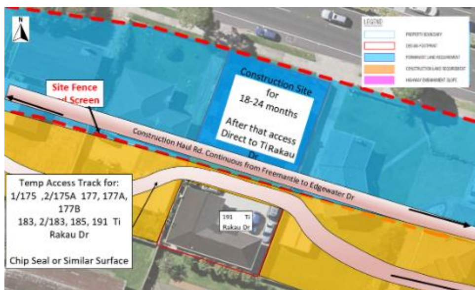
Figure 94: 191 Ti Rakau Dr temporary access
