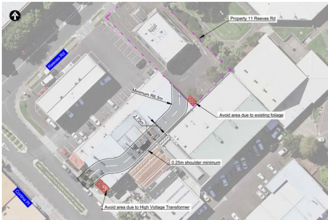
Figure 77: 11 Reeves Rd temporary access during construction
